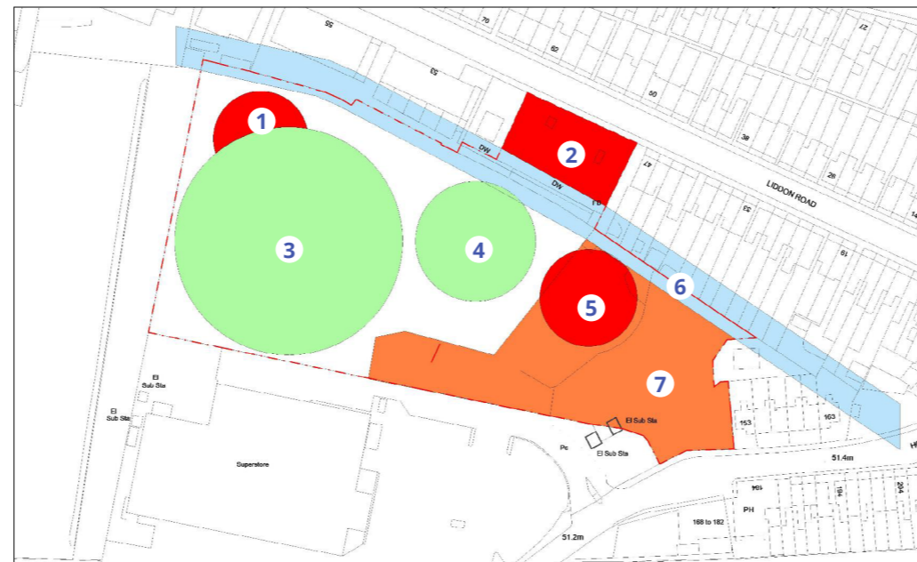
1. Gasholder 3 with high level of contamination - parking possible. 2. Anticipated sludge filled pipes in this area along with other ground obstructions - Open Yard & Parking Possible 3. Gasholder 4 - decontaminated - Residential Possible 4. Gasholder 2 - decontaminated - Residential Possible 5. Gasholder 1 - contaminated fill - Open Yard Possible 6. 8 meter consultation zone either side of culvert. Any significant building within this zone will be subject to a Floor Risk Activity permit with EA 7. Former National Grid Site. No open ground within area due to contamination.
